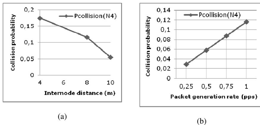
Figure 3. Variation of collision probability for the node 4 according to inter-node distance (a) and packet generation rate (b).
