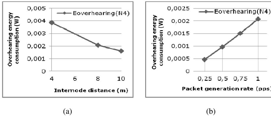
Figure 4. Variation of overhearing energy consumption for the node 4 according to inter-node distance (a) and packet generation rate (b).
