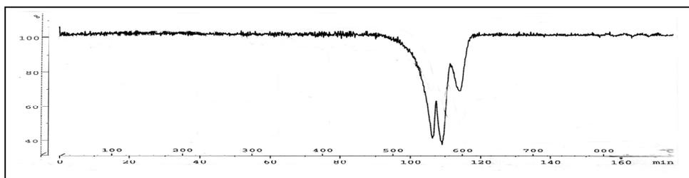
Fig. 11 DTA curve of Fe -doped cadmium iodate
