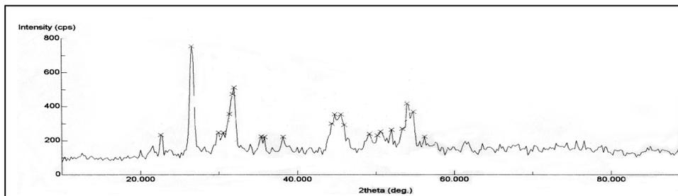
Fig. 4 X-ray diffractogram of Cu-doped cadmium iodate
