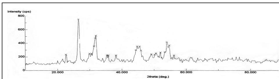
Fig. 3 X-ray diffractogram of undoped cadmium iodate
