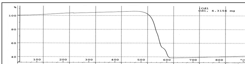
Fig. 6 TGA curve of undoped cadmium iodate
