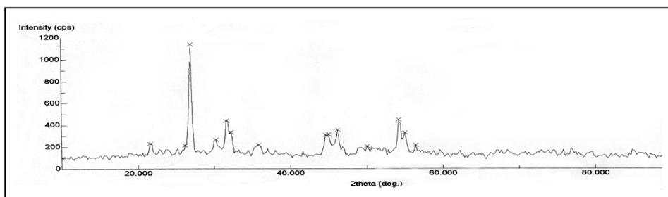
Fig. 5 X-ray diffractogram of Fe-doped cadmium iodate
