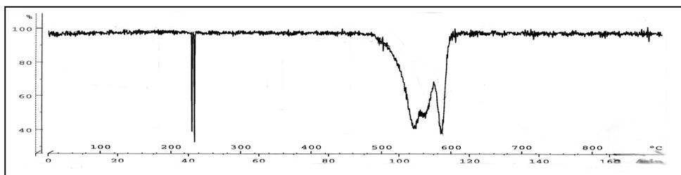
Fig. 9 DTA curve of Cu-doped cadmium iodate
