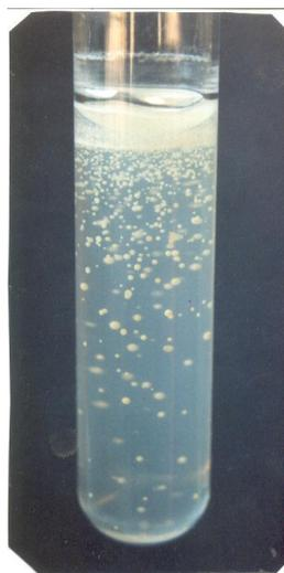
**Fig. 1.** Cadmium iodate crystals grown inside the test tube
