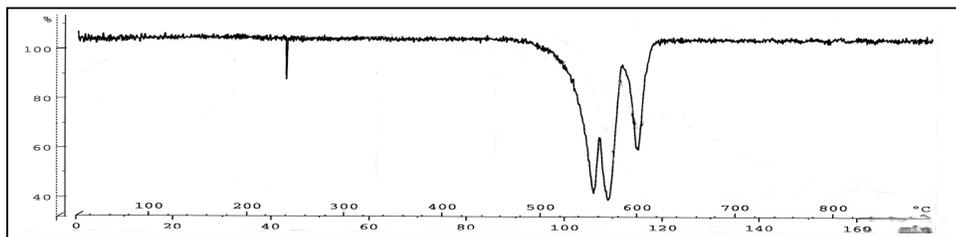
Fig. 7 DTA curve of undoped cadmium iodate
