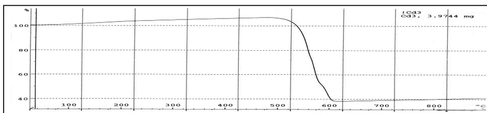
Fig. 10 TGA curve of Fe-doped cadmium iodate
