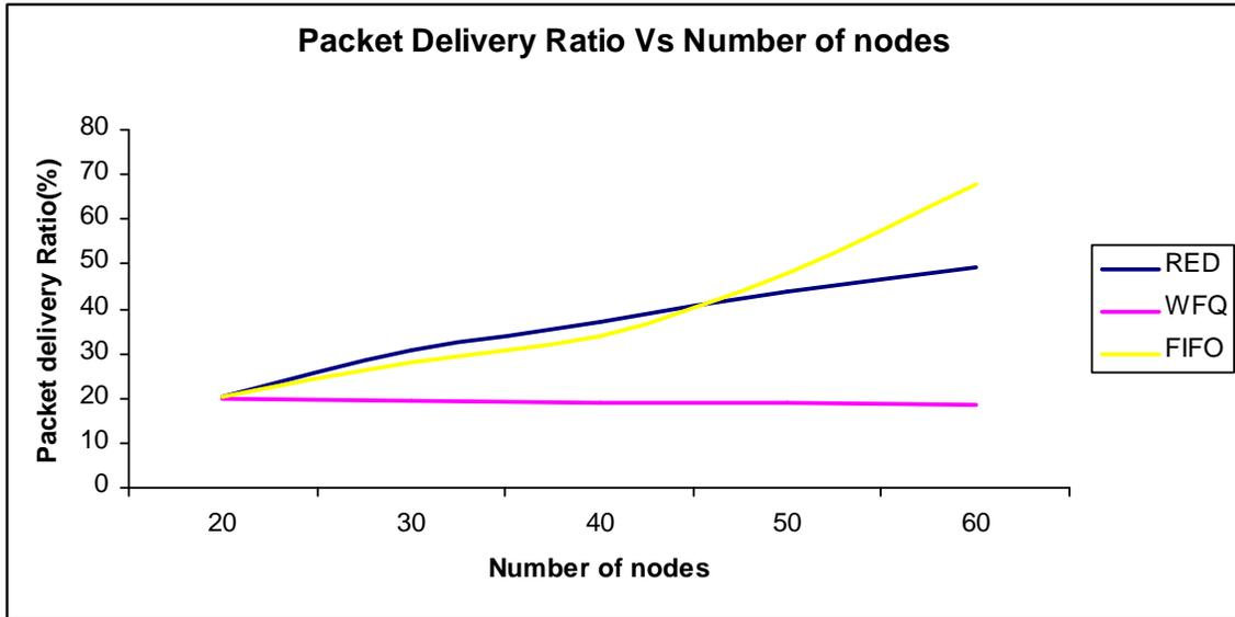
Fig.2 Packet Delivery Ratio Vs Number of Nodes
