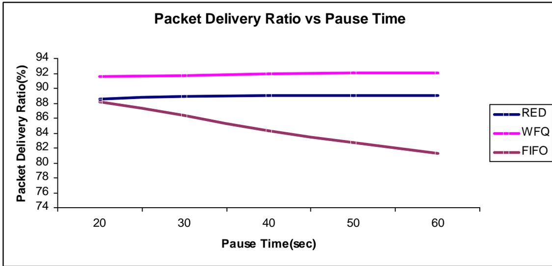
Fig.4 Packet Delivery Ratio Vs Simulation Pause Time
