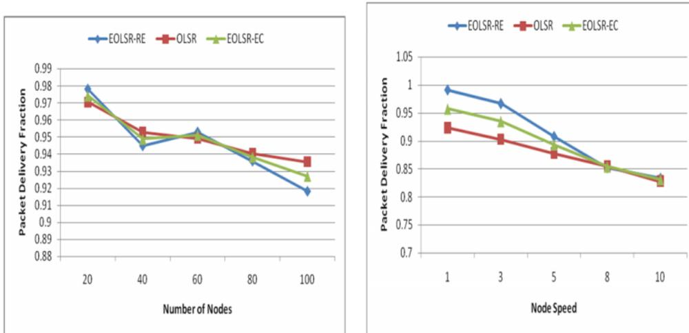
Figure 11: Impact of Variation of Number of Nodes and Node Speed on Packet Delivery Fraction
