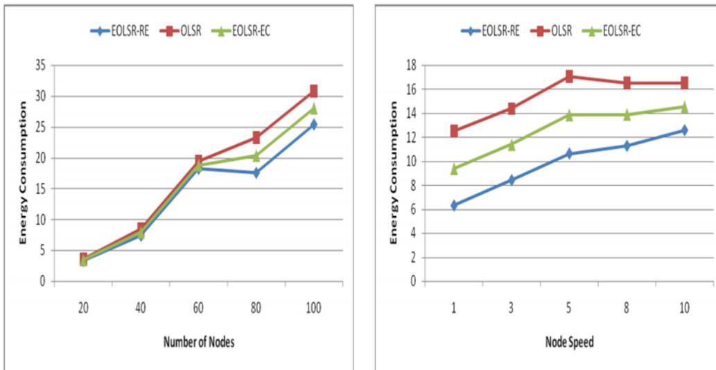
Figure 12: Impact of Variation of Number of Nodes and Node Speed on Energy Consumption
