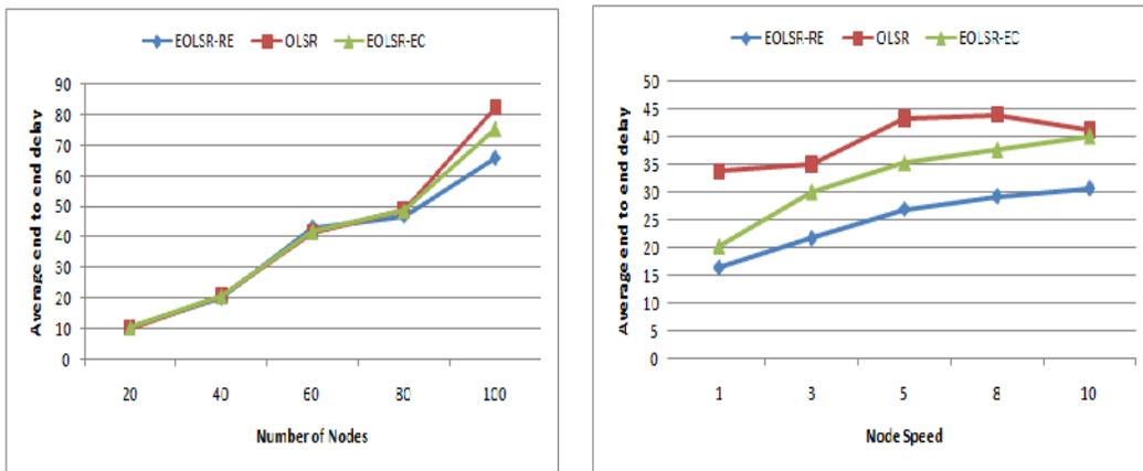
Figure 10: Impact of Variation of Number of Nodes and Node Speed on Average end to end delay
