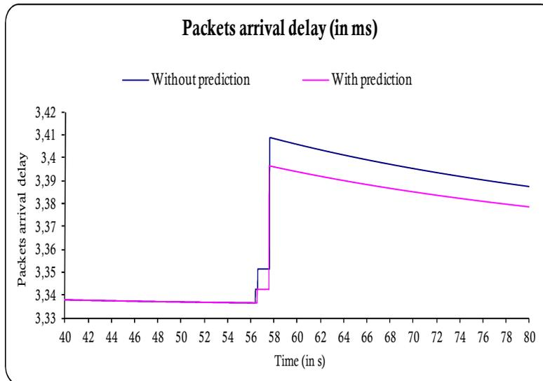
Figure.6. Packets arrival delay vs time for the two scenarios.
