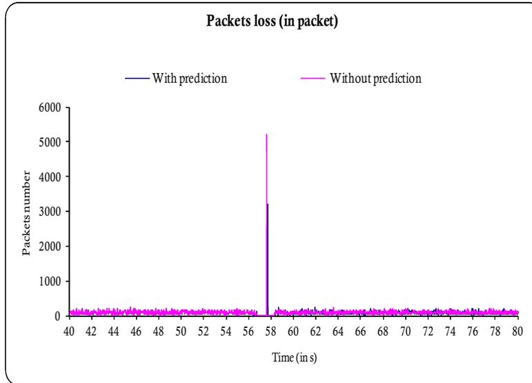
Figure.5. Number of packets loss vs time for the two scenarios.
