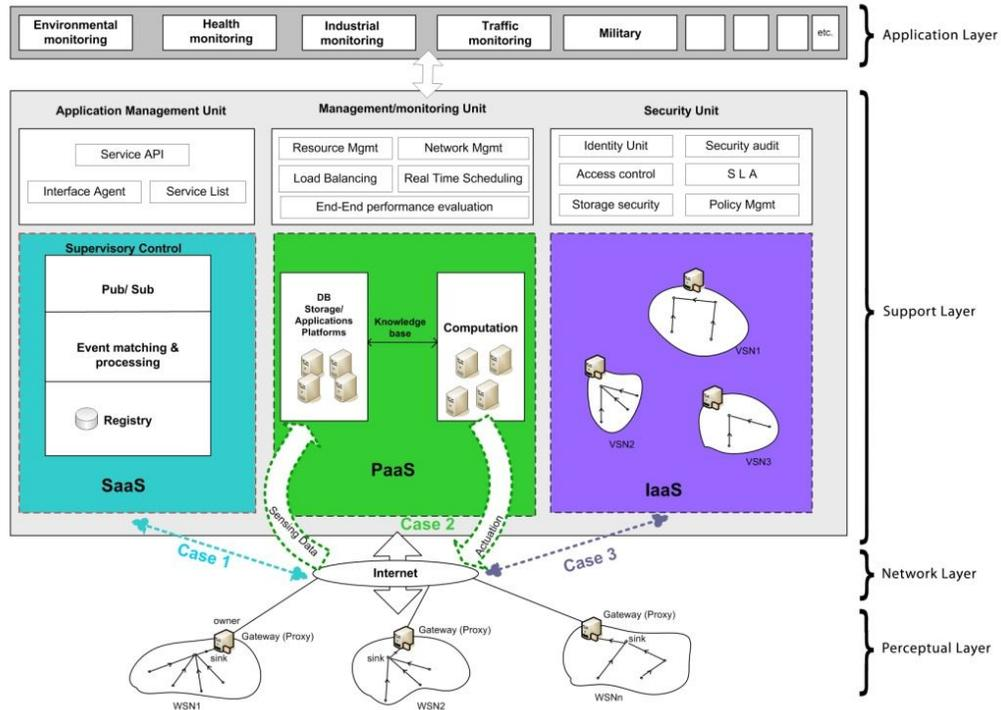
Figure 1. Proposed Secure Service Provisioning Framework for CPCCS: Case (1). Pub/Sub systems as SaaS, Case (2). Sensing and Actuation Systems as PaaS and Case (3). Virtual Sensor Networks as IaaS.
