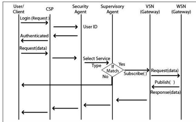
Figure 2. Workflow diagram for the proposed secure service provisioning framework of CPCCS.
