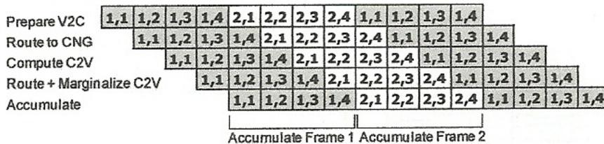
Fig. 5. Pipeline Diagram for rate 1/2, 5/8, and 3/4 codes where the first number indicates the frame and the second the sub-iteration
