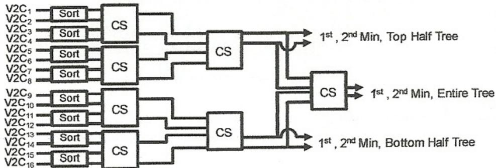
Fig. 3. Check Node Magnitude Computation Schematic
