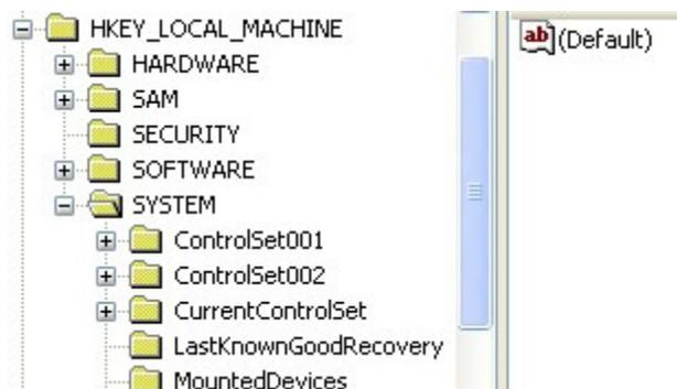
Figure 2. HKEY\_LOCAL\_MACHINE Root Key and Its Subkeys
